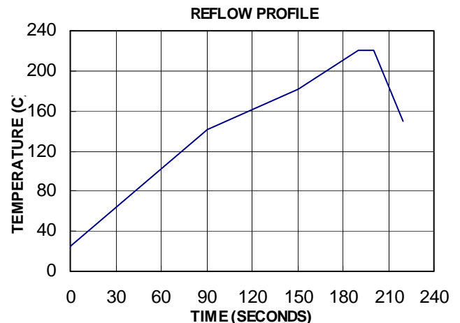
Figure 18 SMT Reflow Profile
